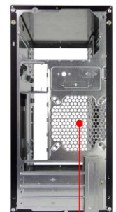
Rear Fan (Optional) 80x80 mm x 1 or 90x90 mm x 1
